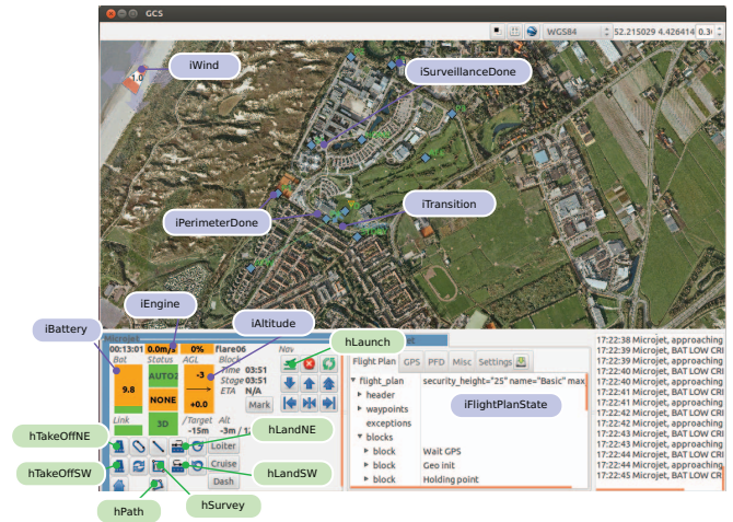
Fig. 2: Links between the EOFM/SAL model and the Paparazzi ground station interface. Model variables are linked to their approximate location for perception of the UAV and ground station output (variables starting with “i”) or their action button (variables starting with “h”).
